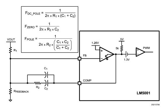
FIGURE 1. Type II Compensator
