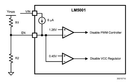
FIGURE 3. Basic EN (UVLO) Configuration
