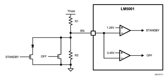
FIGURE 4. Remote Standby and Disable Control
